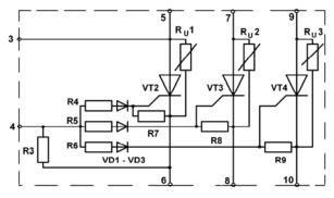
Fig. 11a. Power demultiplexer on thyristors for switch-on the group of trip coil
