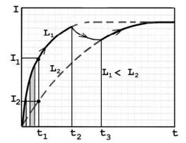
Fig. 1. Dependence of current (*I*) breaking at contacts bouncing during making process from inductance (*L*) of load.  $I_1$  – current breaking at low inductance of load;  $I_2$  – current breaking at high inductance of load;  $t_1$  – bouncing period;  $t_2$  – start moving of core in trip solenoid;  $t_3$  – stop moving of core in trip solenoid
